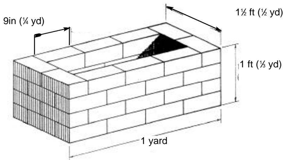
A glance at the next figure, which is the same structure made from 'metric' bricks reveals that these **will not fit a metre**, either lengthwise or coursewise.
